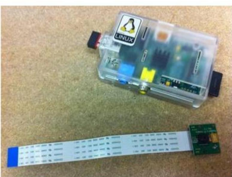
Short description: Raspberry pi technology provides us with low cost and form factor design while still packing the computational punch to do some complex tasks. This makes it an ideal platform to underpin a more advanced spectrometer that has a dedicated camera and processing system. Ideal to work out a spectrometer.
