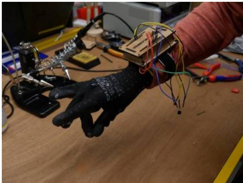
Short description: The participants will build an IRglove that will serve as a remote control for a certain device. By joining two fingertips, a signal will be emitted by the IR emitter to a TV or a radio. A controller and a battery integrated in a bracelet are attached to the glove.
