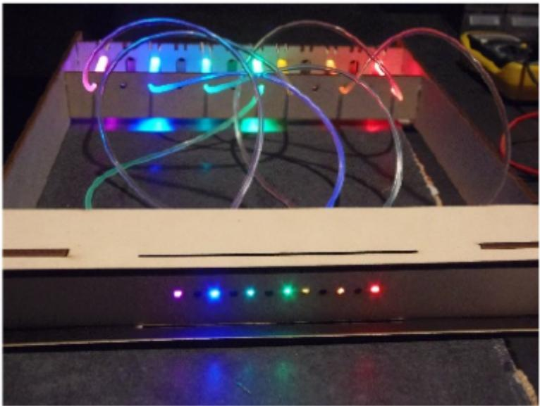
Short description: Optical fibers and music: the Photonics Harp. Each note in the harp will have a different coloured LED connected and aligned to a fibre. When pressing down a fibre, the fibre gets misaligned and the emitted light cannot be coupled anymore in the fibres. The light switching process is coupled with sound. A note will be produced once the corresponding illuminated fibre is switched off.
