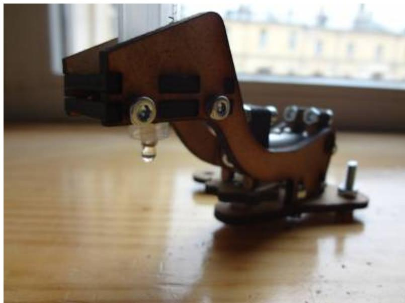
A Droposcope is a simple microscope which uses a drop of water as a lens. The image of organisms inside a water drop is projected on a screen using a laser.
