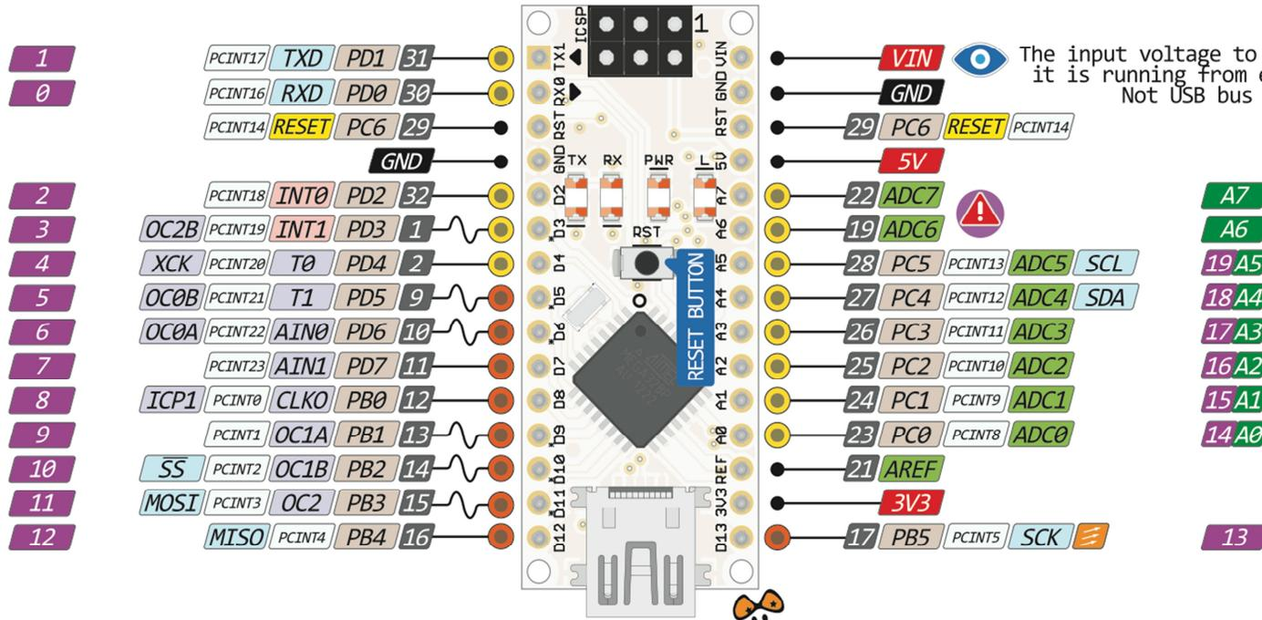
The input voltage to the board when it is running from external power. Not USB bus power.
